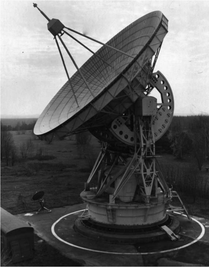
Fig. 1.4 The 22-m radio telescope of the P.N. Lebedev Physical Institute in Pushchino, 100 km south of Moscow. With this instrument, the excited hydrogen line n_{91} \rightarrow n_{90} was clearly detected on 27 April 1964
